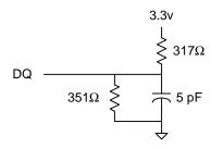
Fig. 2 OUTPUT LOAD EQUIVALENT
