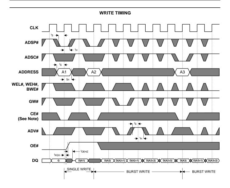
Note: CE# active in this timing diagram means that all chip enables CE#, CE2, and CE2# are active.
