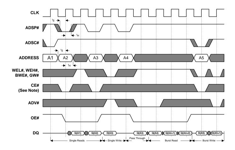
Note: CE# active in this timing diagram means that all chip enables CE#, CE2, and CE2# are active.
